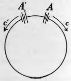
Let us consider two of these accumulators, A and A', inserted with their poles inverted in the same circuit. Suppose they are quite identical, except that the one, A', is entirely without charge, and the other, A, has its full charge. Let us suppose now that the current, c, generated by A which tends to charge A' can under certain circumstances cause an oscillatory discharge, i. e., a continuous oscillation of the current, now in the direction of c, now
